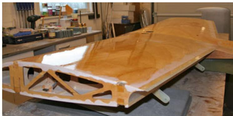
This is the time to coat any exposed areas of un-skinned wood as well, engine bays, wheel wells, fuel tank bays etc.
